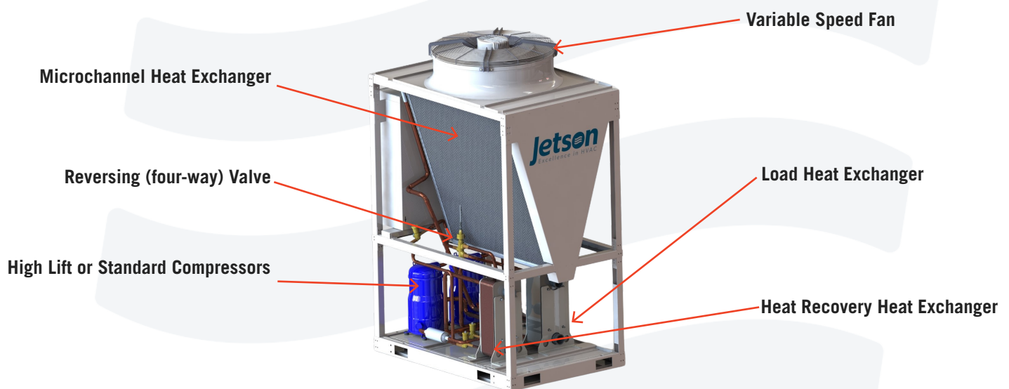
4-pipe Air-to-Water Heat Pump with Heat Recovery Option
