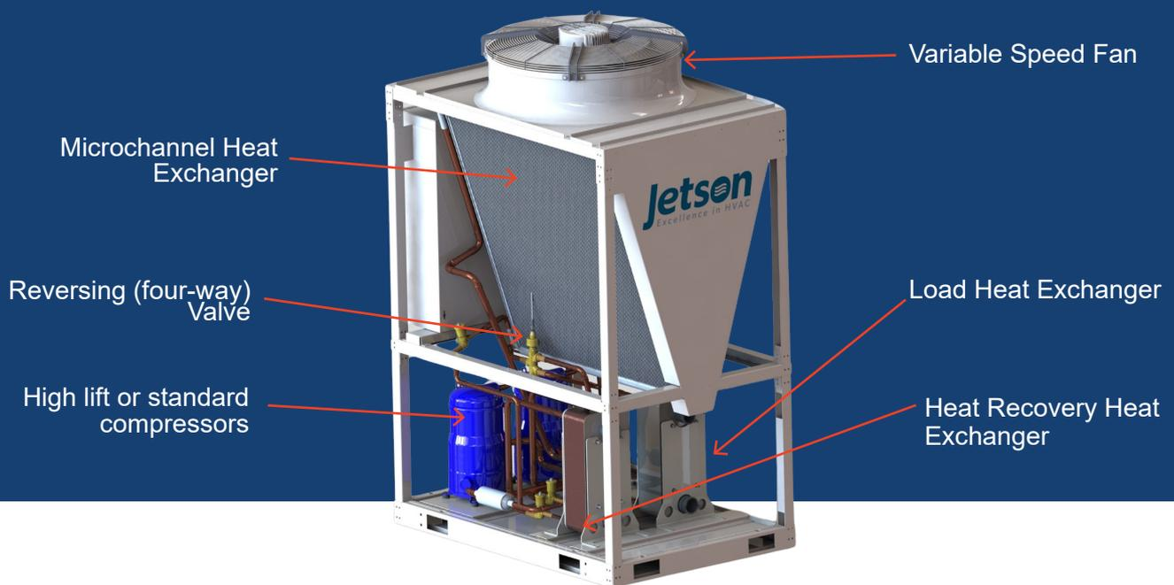
Figure 5. Four Pipe Heat Pump with Heat Recovery
