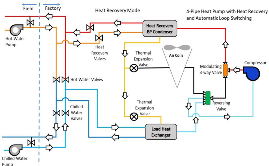
**2. Heat mode** - When there is not a cooling load, four-pipe AWHP units can produce heat, but require additional water piping and valves to separate the heating loop from the cooling loop. Four-pipe AWHP heating mode can be seen in Figure 7. As shown in Figure 7, the refrigerant-to-air heat exchanger is the energy source in the circuit, absorbing heat from the outdoor air, while the refrigerant-to-water is the energy sink in the circuit, rejecting heat to the heating water circuit.
