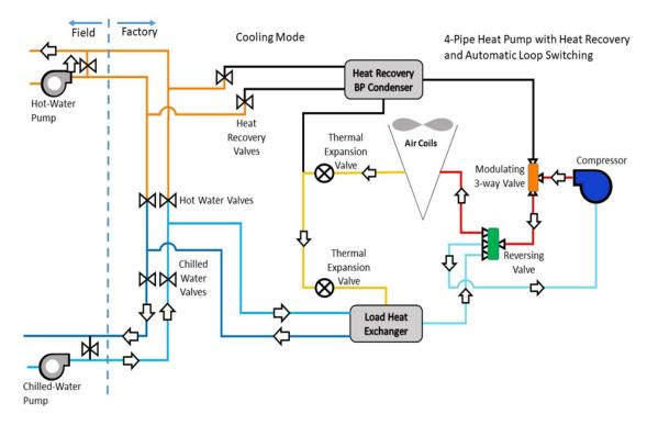
**4. Defrost Cycle** – Figure 9 shows the refrigeration circuit is in the cooling mode supplying heat to melt accumulated ice from the refrigerant-to-air heat exchanger. The return heating water is the source for the heat energy needed to defrost the outdoor air coil. The heat energy for defrost is extracted from the heating water loop.
