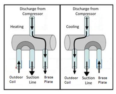
Figure 1. Reversing (four-way) valve
