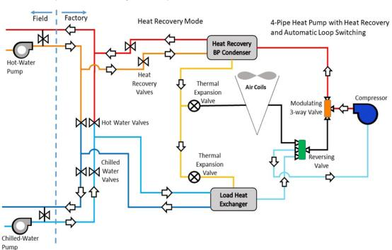
Figure 6. Four-Pipe Heat Recovery Mode Operation
