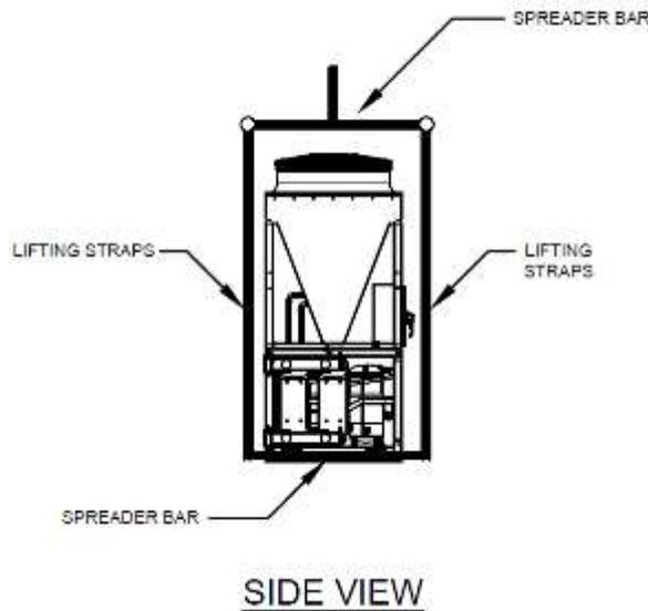
Figure 1 Rigging and forklift pockets
